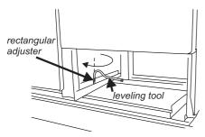
LOWER THE FRONT ROLLER by doing 14 complete (360°) turns clockwise. (This means turning and removing the levelling tool 56 times).
